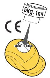
This European Standard specifies physical and performance requirements for industrial safety helmets. Industrial safety helmets are intended primarily to provide protection to the wearer against falling objects and consequential brain injury and skull fracture.
